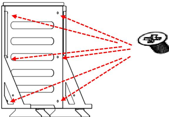
3. Fix the Bracket3 on the back of battery with 4\*Screw2,hook is face down.
