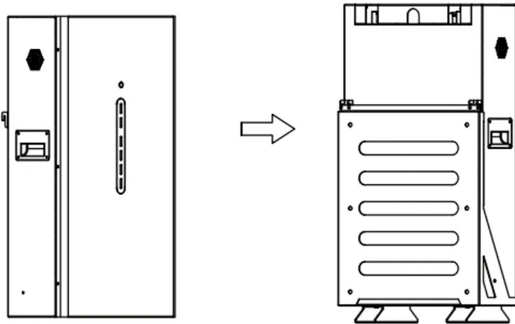
5. Connect the Screw2 on the sides of Bracket1 to fix it with Battery, you can also connect ground cable on the one side.
