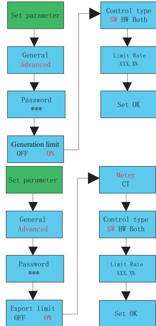
Under the permission given by your energy provider, the ratio of your system output power divided by the rated power of the inverter is called Limit Rate. For instance, if the energy provider only accepts 8kVA/kW from your 10kW system, then the Limit Rate of 10kW inverter is 80.0%.
