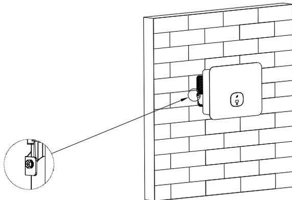
fig5.8 Inverter wall hanging diagram
