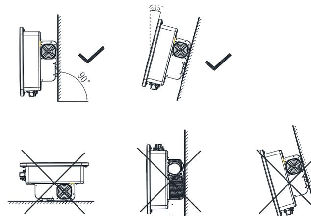
fig5.1 Installation diagram
