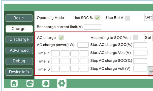
Users can charge batteries with grid power when electricity prices are cheap, and discharge battery power to supply load or export to the grid when electricity prices are high.
