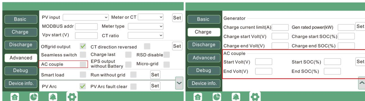
Users need to enable AC coupling function when they connect existing on grid system to GEN terminal.
