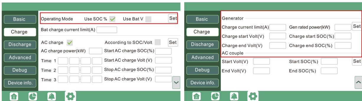
It depends on the Bat operating mode setting, the system will use either battery SOC or battery voltage to determine whether the system needs to start or stop the generator.
