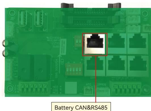
After battery power cable and communication cable connection, users need to enter Advanced settings and choose Battery type and brand on the inverter LCD. After you choose the right battery protocol, the communication will be built in 1-2 minutes.
