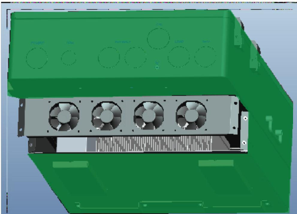
c. Pull out the fan bracket completely, and use a soft brush to clean the fan or replace a damaged fan.
