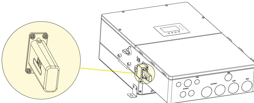
When installing the inverter, make sure that the dongle is connected to the inverter.
