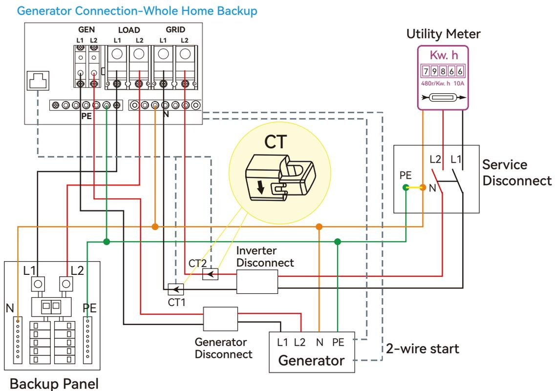
When the generator is started, all the loads connected to EPS Load will be supplied by the generator. Meanwhile the battery will be charged.
