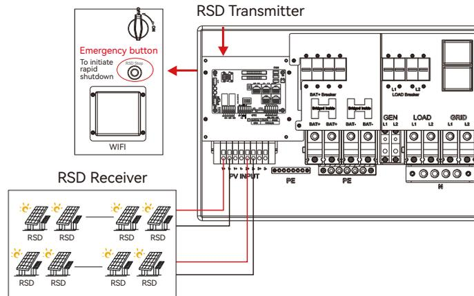
In case of emergency, press the rapid shutdown button that cut off the RSD power supply, thus stopping the inverter AC output, and the PV conductors voltage will be reduced to less than 30V within 30 seconds.
