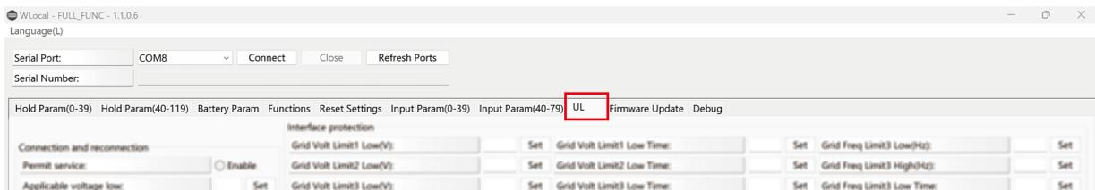
3. In this page, can activation the Rule21 function. Setting the value in the corresponding blank. Before setting, you can read the default value first, and then set the parameter of the function that needs to be modified according to the parameter setting range provided in the next chapter 8.2.
