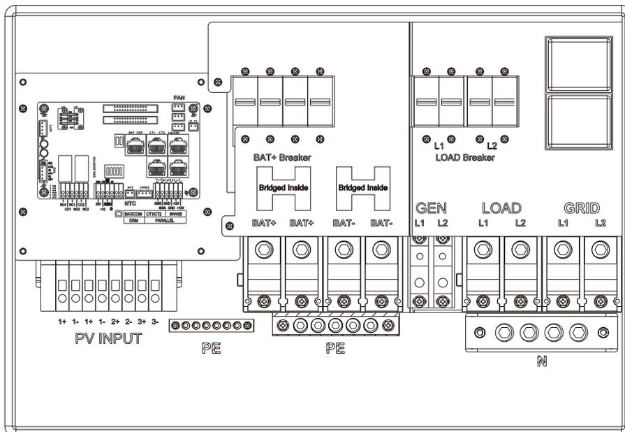
The inverter has integrated Load breaker and BAT breaker, and the Load breaker is 200A, the BAT breaker is 2x200A.
