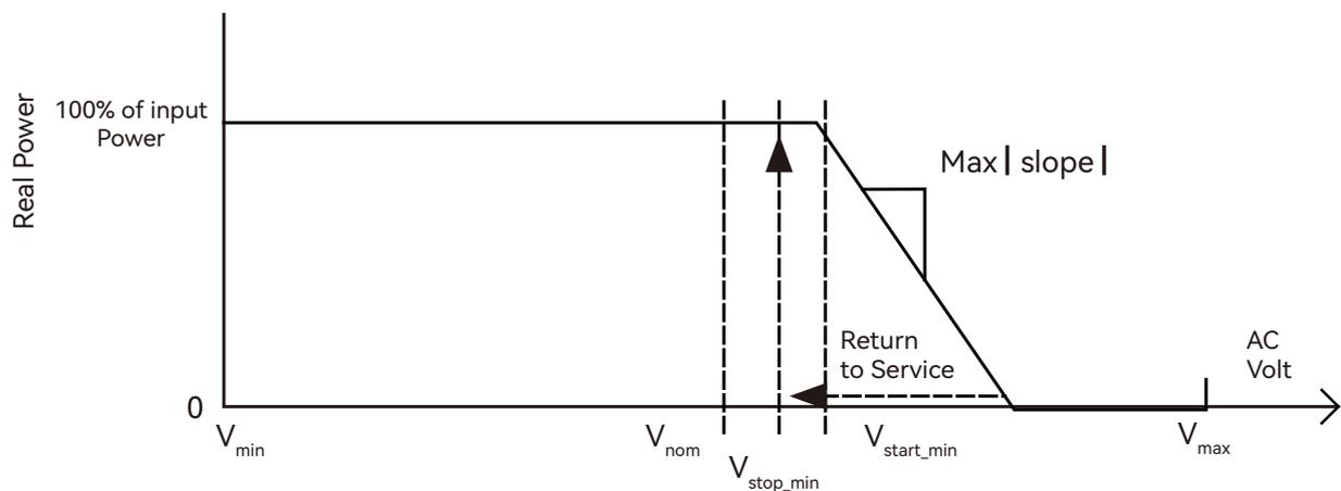
When the grid voltage exceeds V1, the output active power varies with the grid voltage.
