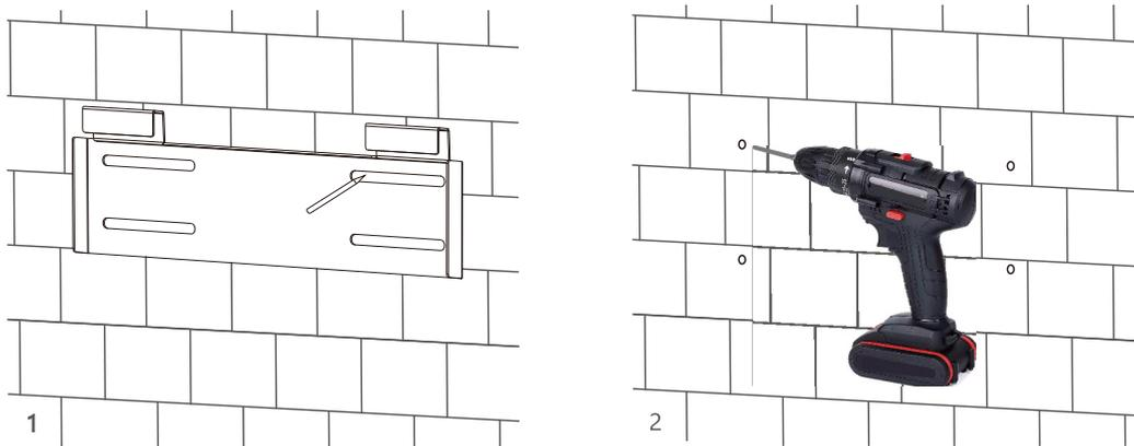
**Step 2.** Install and tighten the expansion bolts into the holes. Then use the corresponding nuts and washers (packaged together with the expansion bolts) to install and fix the wall-mounting bracket on the wall.
