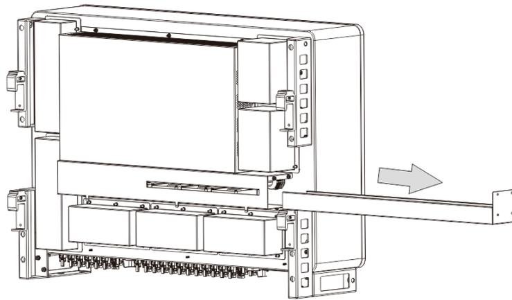
5. In the reverse order as above, reinstall the maintained fan back to the converter and restart the system
