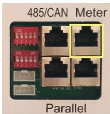
Rj45 Terminal Configuration of Meter/CT Communication
