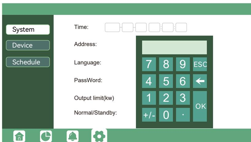
After selecting the corresponding value, click OK, and the number box will be automatically hidden to complete the value input.
