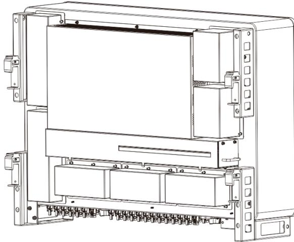
3. Pull the fan tray out slightly until the fan power connector is exposed, press down on the protrusion of the fan power connector and pull it out.
