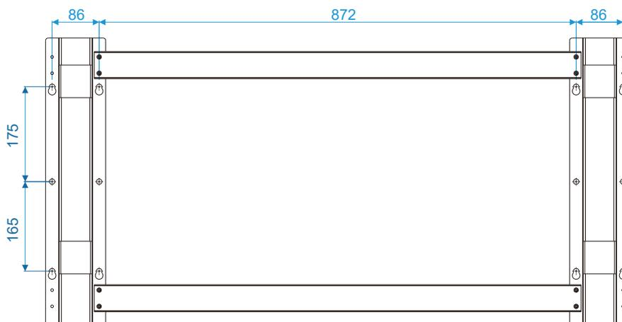
**Step 1.** Install the wall mount bracket. Use the wall mount bracket as a template, drill holes on the wall according to the position of the screw holes on the wall mount bracket, and insert expansion bolts.
