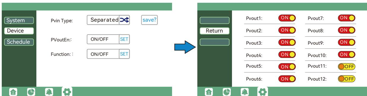
The function options in this navigation column are turned on and off for debugging. Please turn them off carefully, otherwise it may cause the machine to run abnormally or be damaged. Click "return" to return to the previous menu.
