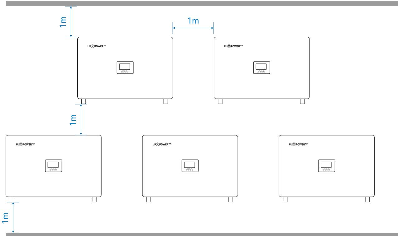
3. Do not install the converter in a closed and small space, as shown in the picture below:
