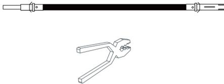
3. Assemble the cables into the positive and negative connection terminal shells to ensure a firm connection
