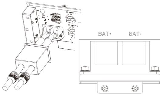
6. Tighten the sealing nut of the waterproof head
