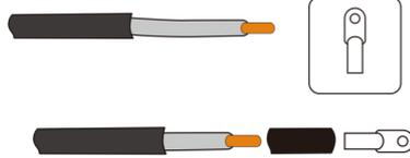
3. Press the DT terminal sleeve wire barrel with hydraulic pliers to ensure that the wire and the terminal are firmly connected
