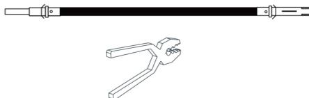
3. Assemble the cables into the positive and negative connection terminal shells to ensure a firm connection
